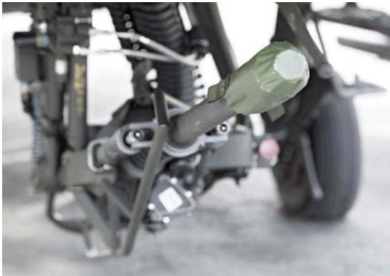
▼ 30MM CHAIN GUN The Hughes M230 chain gun can fire 625 rounds per minute, fed from a 1,200-round magazine by an electrically driven chain mechanism.
